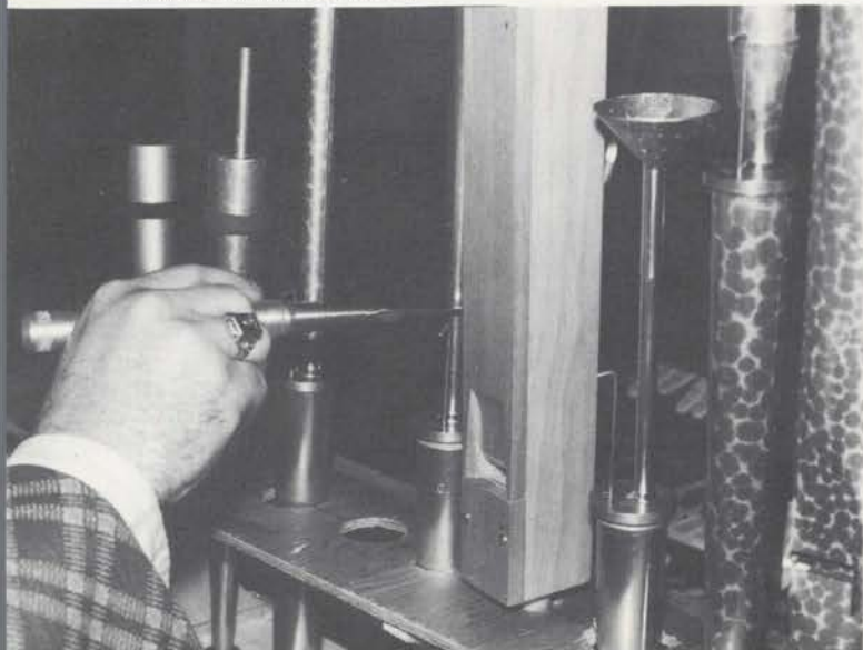
Setting a reed pipe to pitch.
