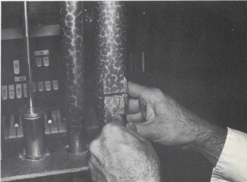
Adjusting the wind sheet of a new Diapason.
