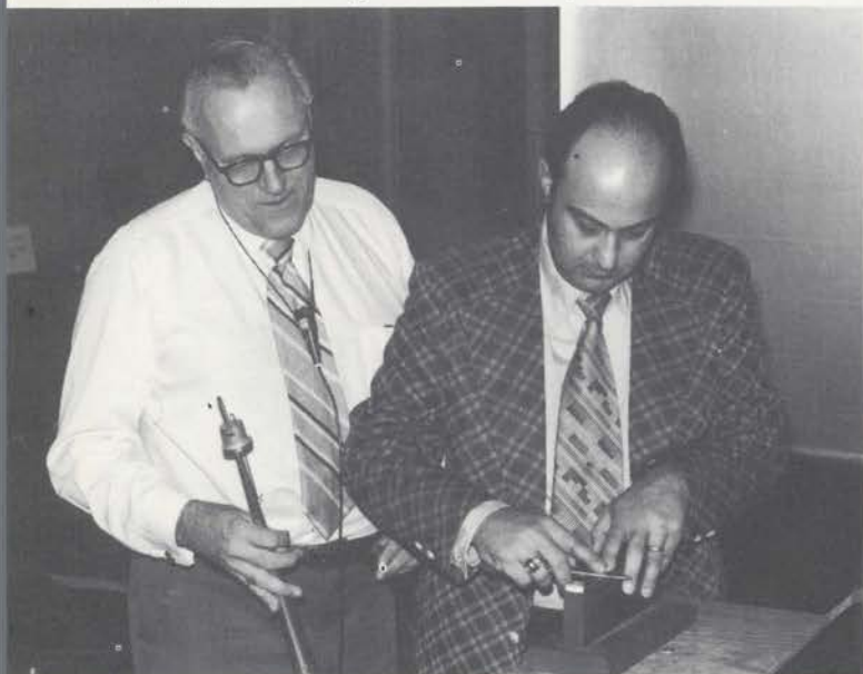
Applying curve to tongue of French Trumpet.
