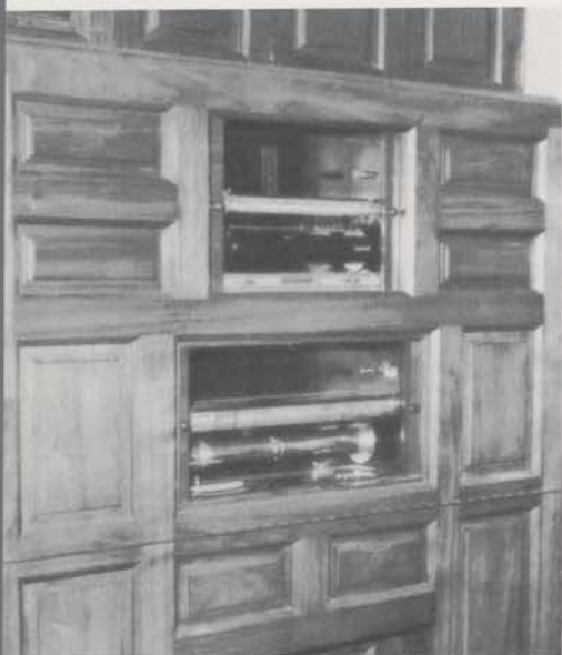
Automatic player actions for both Kilgen and Duo-Art player rolls.
