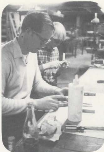
Phil Felde and son recover pneumatics at Johnson Organ Co. plant for Fargo project.
