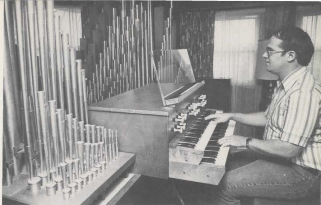
Even the console is mounted on the chest. It took some getting used to being so close to the pipework. The pipes in the foreground are part of the reed Dulzian rank.
