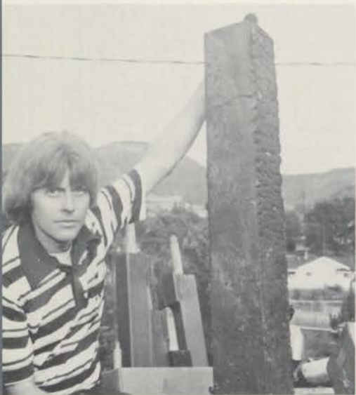
The strain shows on John Ledwon's face as he examines a Tibia pipe burned beyond repair.
