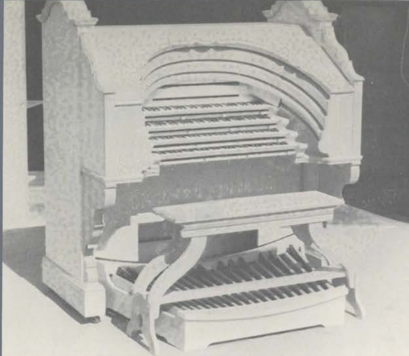
The four-manual Publix French style console built for the residence of Carl Weiss, of Weiss and Turney Pipe Organ Builders, Long Island, N.Y. It will accommodate 315 stop tabs and can control a 40-rank pipe organ.
