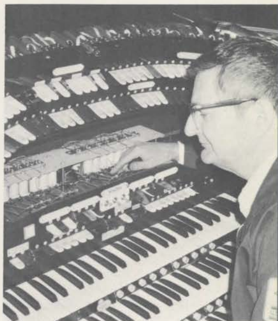
Don Campbell inspects the Wicks action magnet system on the backboard. The toggle switches and indicator lights are also new.
