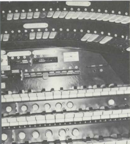
Located just above the trem stop tabs is the selector toggle switch (center of photo) for the Solo Tibia tremos.
