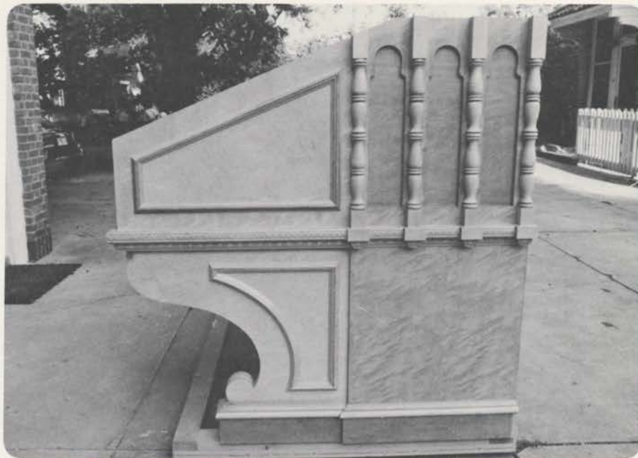
Dr. B. D. Rhea turned the posts for his reproduction of a Wonder Morton console on his workshop lathe.
