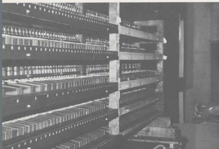
One of the manual chests during rebuild. Note the use of sponge neoprene gasket material.
