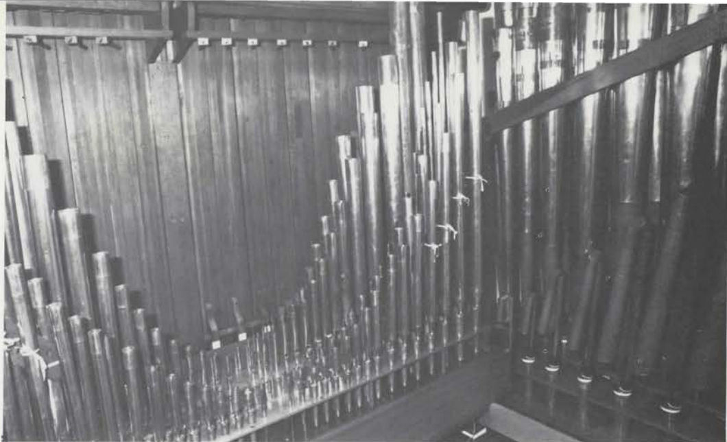
Partial view of Main Chamber showing from front to back: Clarinet, Viol Celeste and Open Diapason, with 16' Tuba Profunda offset on right. Not visible behind the Open Diapason are the Viol d'Orchestre and Concert Flute.
