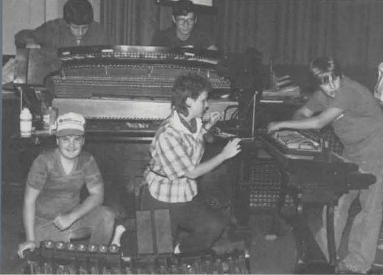
Cleaning is a continuous process for the Wurlitzer, and willing students are always available for the work. Here (behind the console) Mike Brooks and Paul Girouard, seniors at Berlin High School, assist eighth-grader Scott Gallant, teacher Nancy Joy and student Randy Grondin. Randy took the responsibility for replacing the backrail pneumatics, and Scott did most of those on the console. Mike and Paul have been instrumental in training the younger students to be organ "technicians." Jim Martin is justifiably proud of this Wurlitzer and of the work his students have done to restore it to concert condition.
