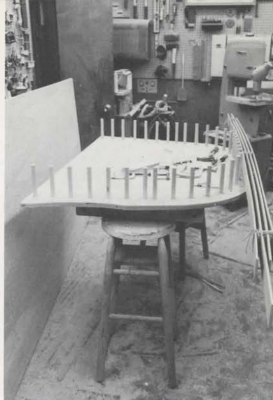
Form which held steam-heated boards for stop bolsters.
