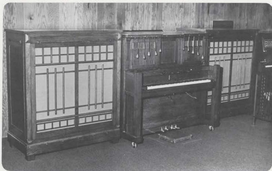
Style 25 American Fotoplayer, used for silent movies. Trap pulls operate (L to R) sleigh bells, train whistle, tom tom, bass drum, cymbal, Chinese crash cymbal, pistol shot, wind, bird whistle, trolley gong or cathedral chime. Side chests also contain three ranks of organ pipes and other sound effects. (John J. Young Photo)
