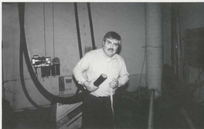
Mike Coup, head of Wichita Theatre Organ, Inc. holds original Wurlitzer cable in right hand and Devtronix flat ribbon cable in left. The small cable replaced the wrist-thick cable when the Devtronix computer relay was installed in the big 37-rank instrument. (Devtronix Photo)
