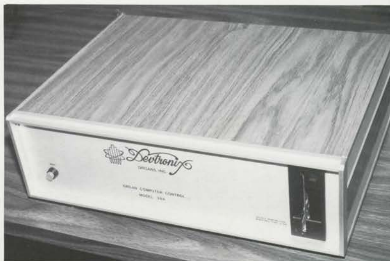
This is the computer unit that replaces cumbersome, heavy relays in the Devtronix computer relay system. (Devtronix Photo)
