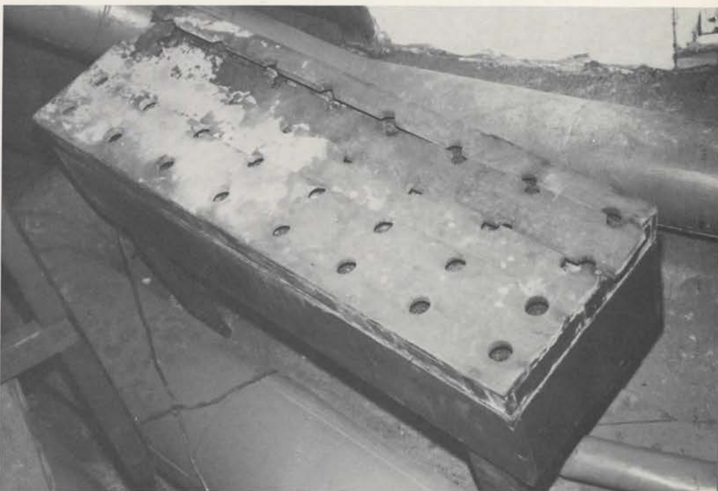
Tremulant shows water damage, an example of the condition of the entire organ before restoration.
