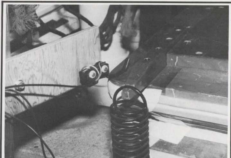
Photo 7: Counter trigger-switch for determining tremolo frequency.
