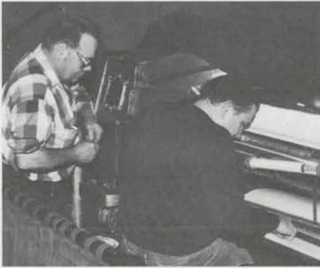
Oren Walther uses a wire wrapper to reconnect cable to new contact springs on the Redford's accompaniment manual Bill Vogel Photo
