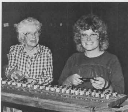
Linnea Kindig and Debbie DeCaro removing old leather and rebuilding magnets.
