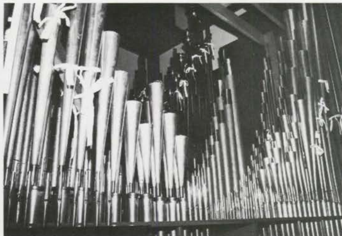
Special scale Post Horn built by Trivo for 17' wind.
