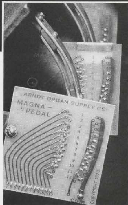
Clockwise from top: Pedal keying diode boards, turned on by magnetic switch on underside of board.
