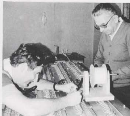
Cumberland Valley members Dean Faulk (left) and Gil Singer wiring new magnets for the Main Chest of the Solo division.
