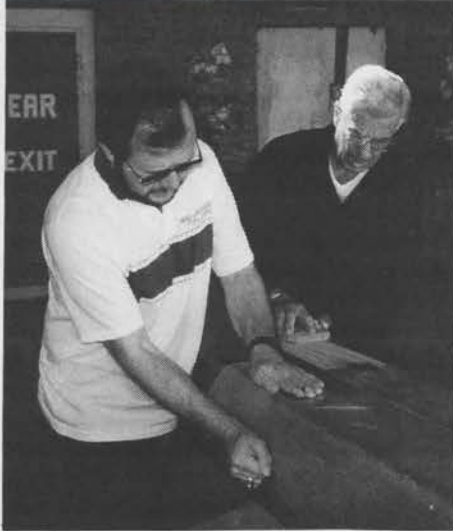
Jim Harland (left) and Gene Mignery refinishing Pedal Flute pipes.
