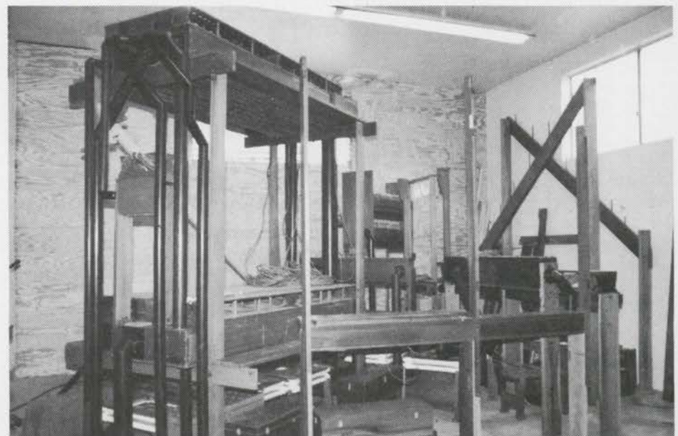
The organ was completely assembled in the Crome shop (except for pipework) so everything fit perfectly in the Sexson chambers.
