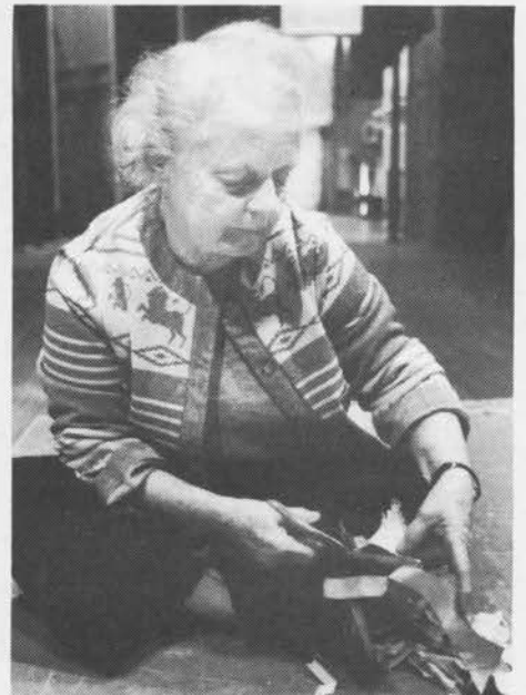
Marion Robere cuts leather strips to seal wind trunks. Chattanooga News-Free Press, Amy Miles Young photo
