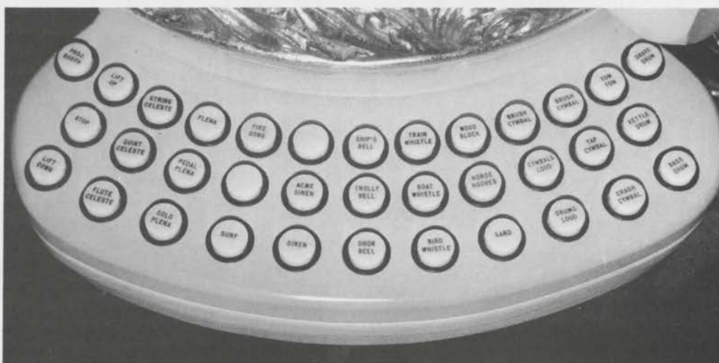
Left swingout shelf, containing buttons for projection booth signal, left controls, celestes off, Tibia Plena stops, and traps. All buttons are reversible, and can be controlled from combination pistons.
