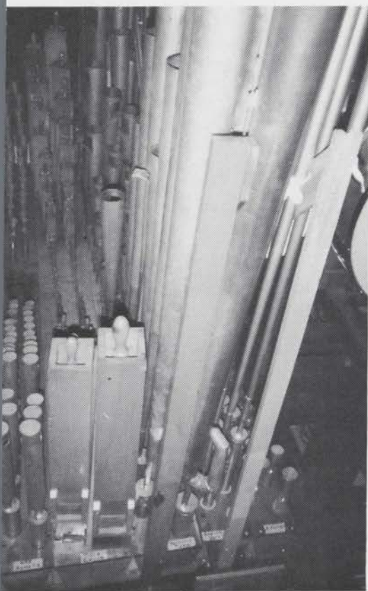
Style 216 Solo Chamber. L to R: Vox Humana, Tibia Clausa, Harmonic Tuba, English Horn, and Orchestral Oboe — though this example has a Kinura in place of the Oboe. Most often when a 216 can be found, it is the English Horn and Oboe which are likely to be missing. DeLay photo
