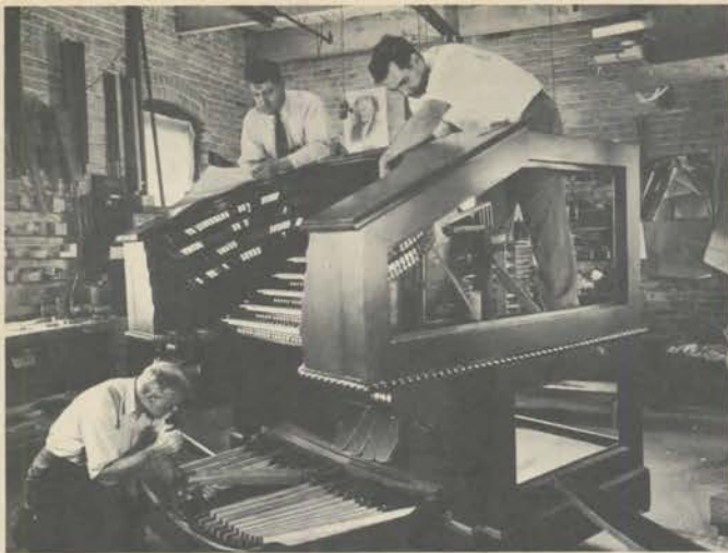
5-manual console nears completion in Moller factory. — Photo courtesy M.P. Moller, Inc.
