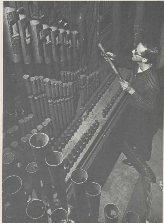
A Vox Humana in the Right Chamber gets Hall's attention. On the chest in front of him are the Kinura, Vox with off set trumpets behind that and in the foreground.
