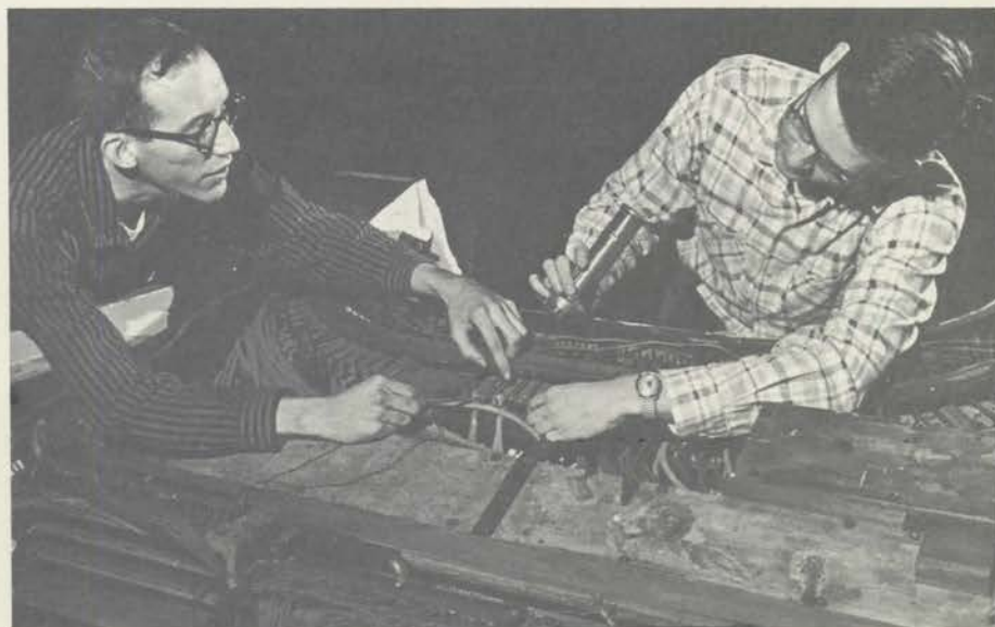
The organ technicians work over one of the pneumatics inside the console.
