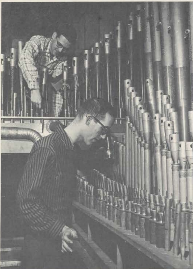
Ross takes his turn at tuning a Trumpet while Hall asks one of the Kinuras to say "Ah." Entrance to this chamber is gained by sliding between the Diaphone resonators and under the Right wind chest.
