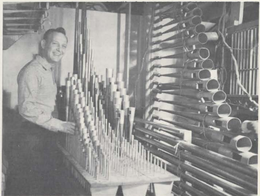
When Tubas and Strings are too high for the ceiling, install them horizontally! View in Main Chamber.
