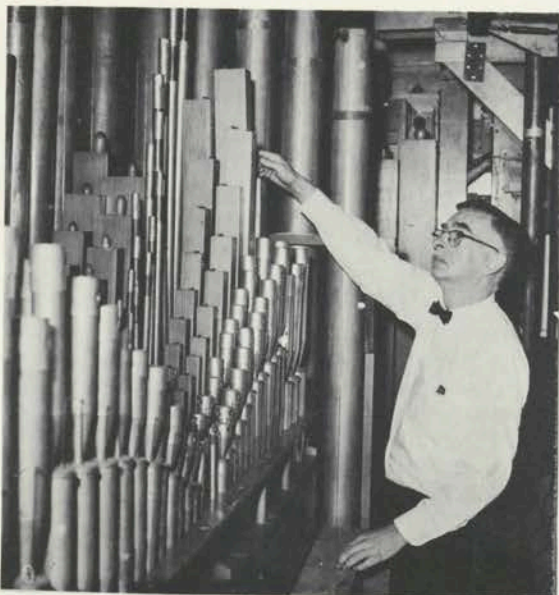
IT'S COOLER INSIDE - Editor George cools his pinky over the exhaust from a ciphering Flute pipe. This photo, shot with a 'nostril' camera, shows some of the instrument's pipe-work. Front to back: Vox, Concert Flute, String, and Tibia. The offset bass Diapason and Tibia are at George's right. There's a bass drum way up there. Swell shutters are directly behind the old grouch.
