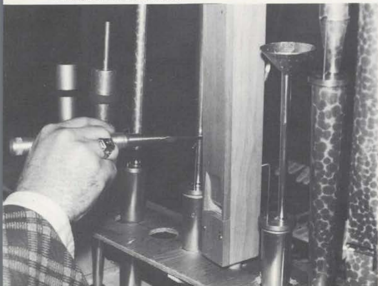
Setting a reed pipe to pitch.
