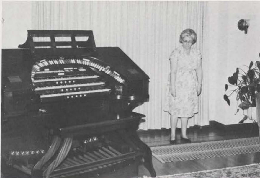
Mrs. Burke points to the grillwork in living room floor, where the organ speaks from the basement chamber.
