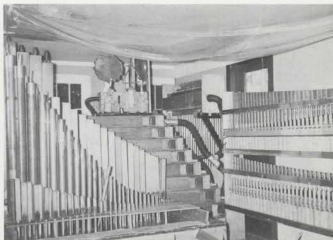
Above. Some of Jon's pipework, percussors and toy counter as installed in the Fennville home. Note the horizontal installation of the bass flute pipes — pit organ style.
