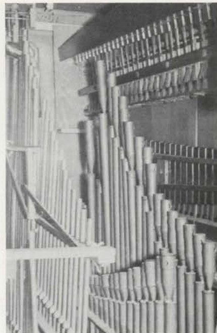
The original 49-note String and Vox ranks and the original Xylophone (right). The added Glockenspiel is at upper right.
