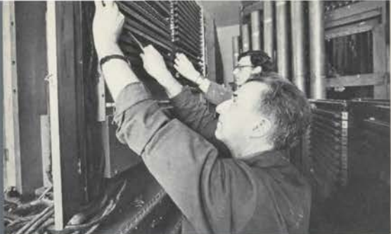
Ken Hodgson, supervisor of Wurlitzer rebuild, with assistant Bert Blok putting final touches on the complex switch stack system.
