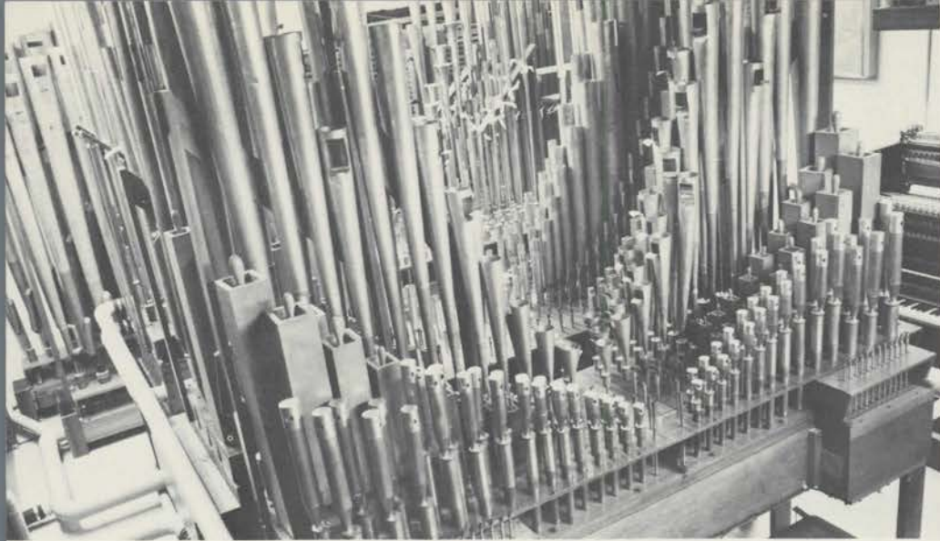
General view of pipework. Note careful placement of windlines.
