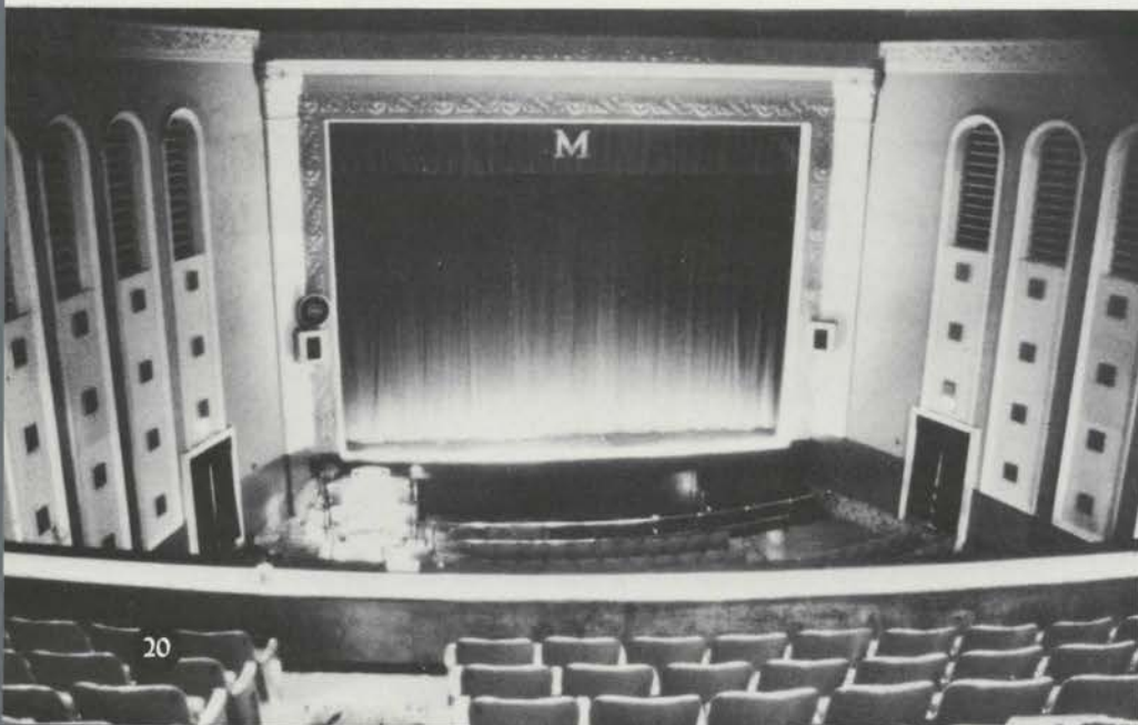
The 3/13 Barton is on a four-poster lift at the left corner of the orchestra pit. The organ speaks through the grilles on either side of the auditorium.
