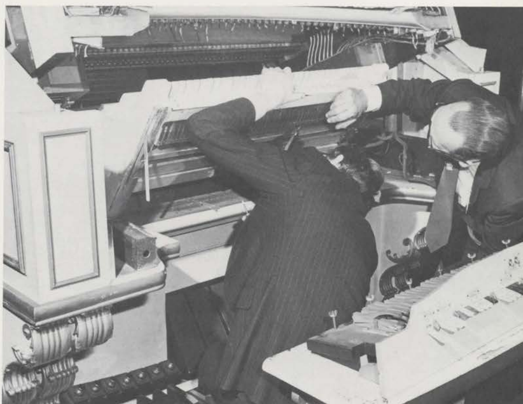
Len and Les Rawle repaired the faulty key contact and reassembled the console in record time.
