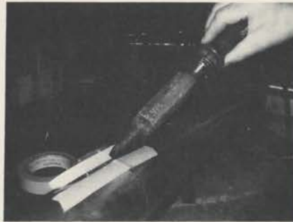
Using masking tape to protect pipe metal while soldering on an ear.
