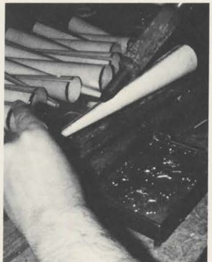
"Drawing" a bead of solder down the seam.
