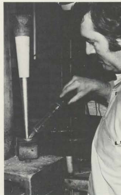
Soldering a resonator onto a reed block. Note fixture used to hold resonator perpendicular to block.
