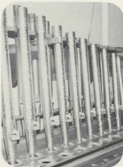
Newly fabricated set of Quintadena pipes, still on the voicing machine. Getting the voicing right is a Miller specialty.
