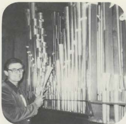
A pleased Bill Brown examines his new rank of Tuba Mirabilis pipes, a precision re-creation of a Wurlitzer set.
