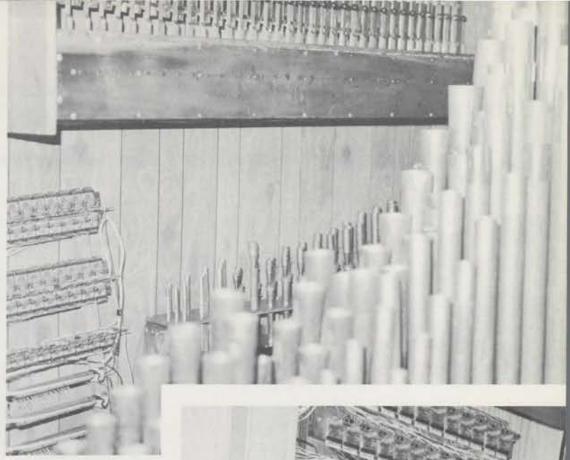
Top Left — Although not original Wurlitzer, the toy counter looks and functions much like those made years ago. Made by Gorsuch Enterprises, it was ordered "with room to grow."
