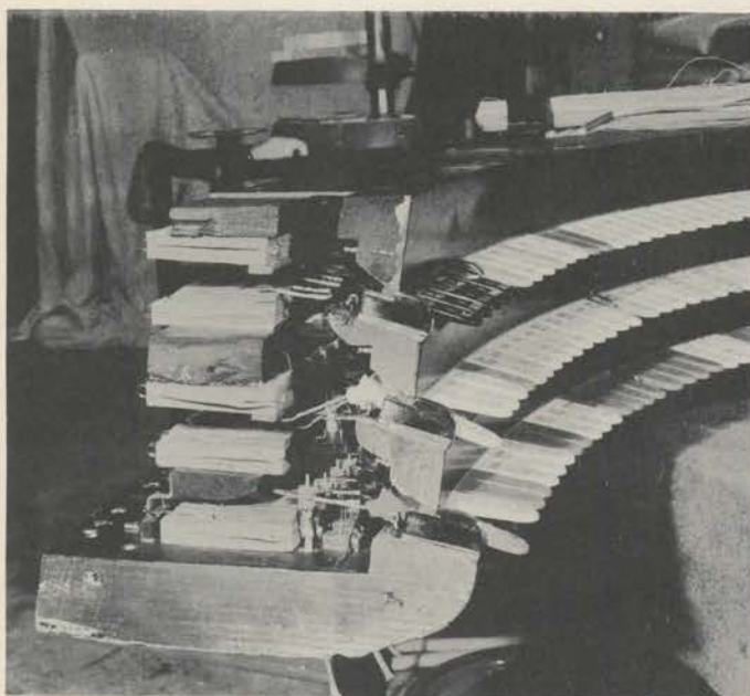
Close-up of Bolster showing three tiers of stops and pneumatics, specially built from Wurlitzer plans.
