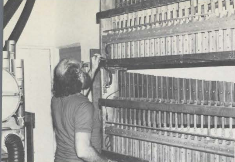
Bob Garner checks out the reiteration relay which was added to the orchestra bells.
