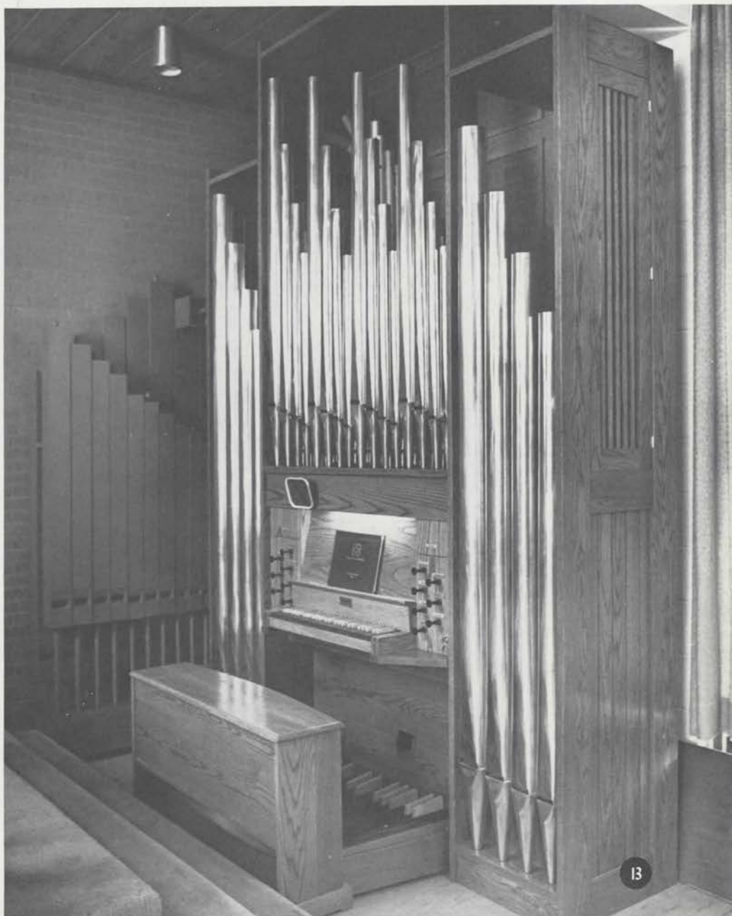
Below: The 1/8 tracker-action organ built by the Johnson Organ Company for the Dilworth Lutheran Church. The facade contains polished aluminum pipes from the Spitzflöte. The case is made of red oak; manual keys have rosewood naturals and hard maple sharps. Manual stops divide at tenor B/middle C. The pedal rank, located at the left side of the case, uses electric action.
