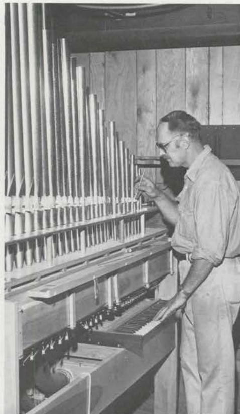
Lance working at tracker voicing machine.
