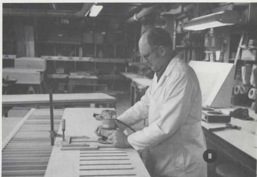
Routing pallet slots in pallet and slider chest. Johnson Organ Company uses this type of chest on all their church instruments.
