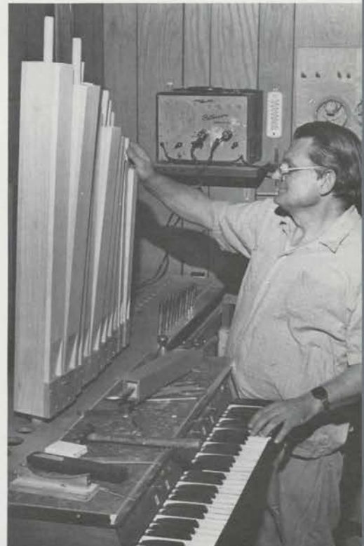
Head Voicer Craven Nichols at the voicing machine. Old Peterson tuner on wall is wired into voicing machine to facilitate rough tuning.
