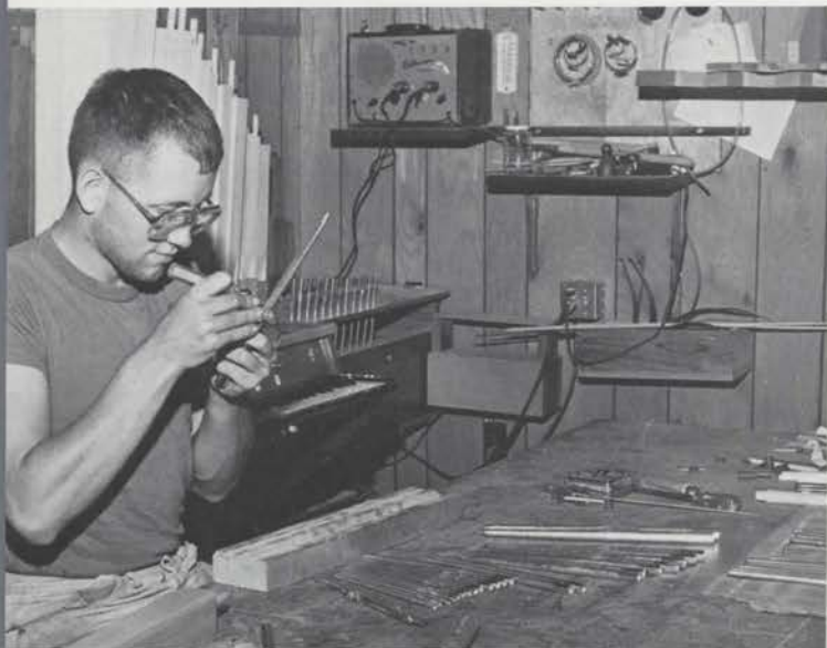
Lance's son, Mike, preparing low pressure principal pipes for voicing.
