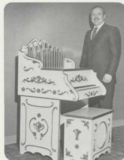
Matt Neill and his electronic calliope. The speaker is in the bench. (Claude Neuffer photo)
