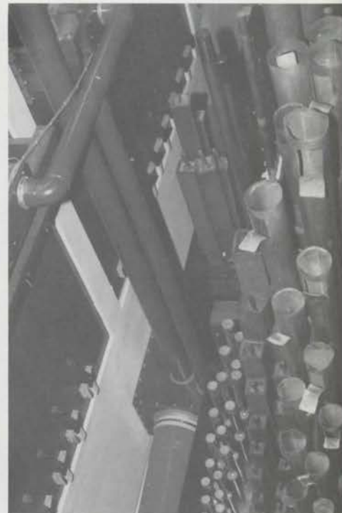
Two views of the Main chamber, showing pipework and wind lines.
