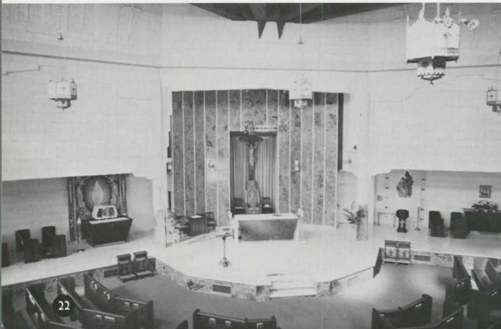
Looking down from balcony. Hard surfaces are behind altar, tile floor around altar and the side wings. The aisles are carpeted.
