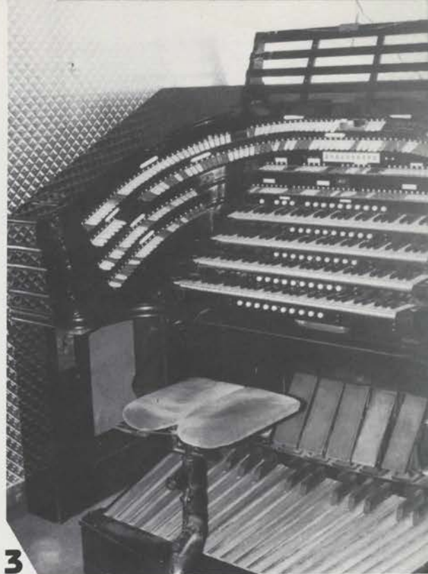
3 Right console of the 4/58 Wurlitzer. Note hole on left side under key desk.
