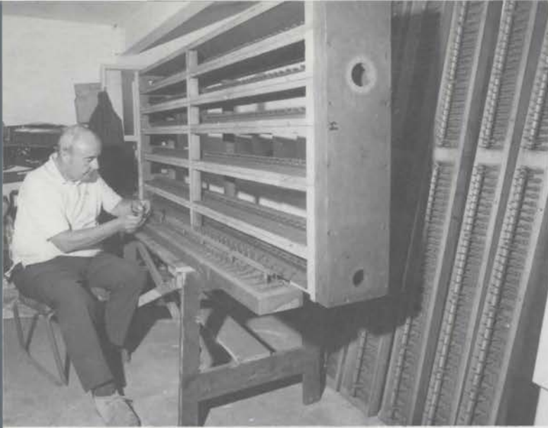
Eric Penney releathering the six-rank chest from the Solo chamber.
