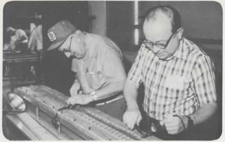
Central Indiana members Dusty Desterbecque and Dave Ketcham refurbishing wind chests at Manual High School "work party." (John W. Ennis photo)
