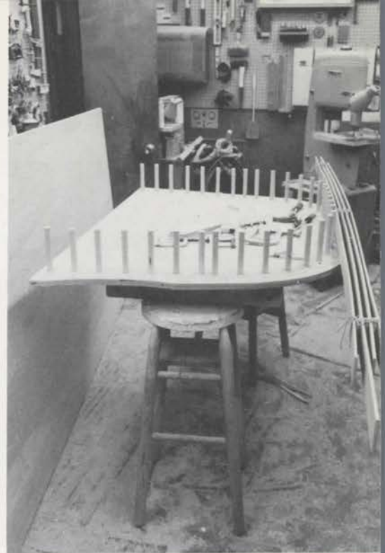
Form which held steam-heated boards for stop bolsters.
