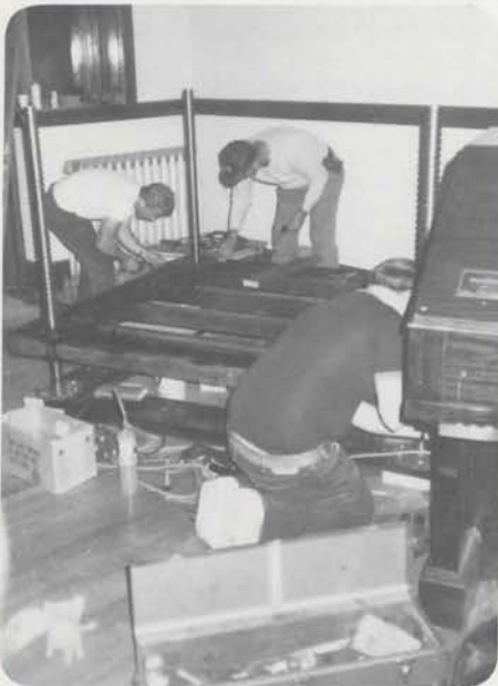
Members Keith Roberts, Gene Mignery and Ken Davies rebuilding the four-poster Barton lift for the Pikes Peak chapter Wurlitzer at Mount St. Francis.
